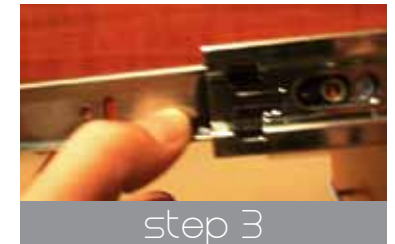
step 3 For slide on right side of drawer box locate the black tab and push DOWN to release. With both tabs released at same time slide out the drawer.
